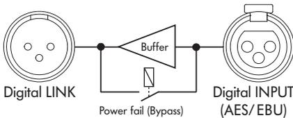
**Fig. 15: D12 Digital INPUT Bypass**
